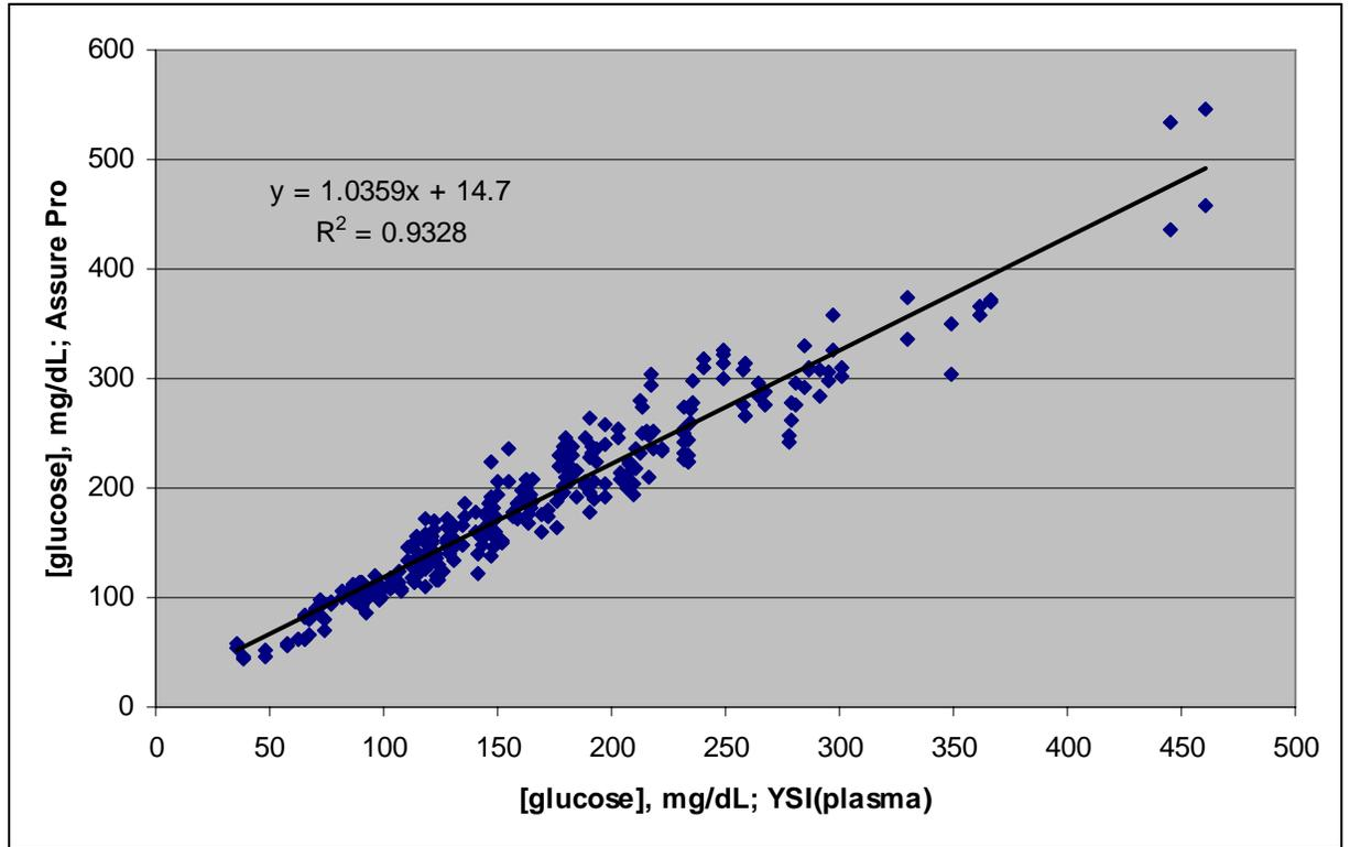
The following graph illustrates the performance of device when used by a lay user as compared to a laboratory reference:
